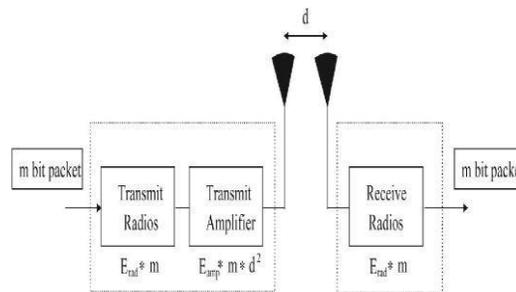
**Figure 3: Energy dissipation model of the proposed scheme.**
